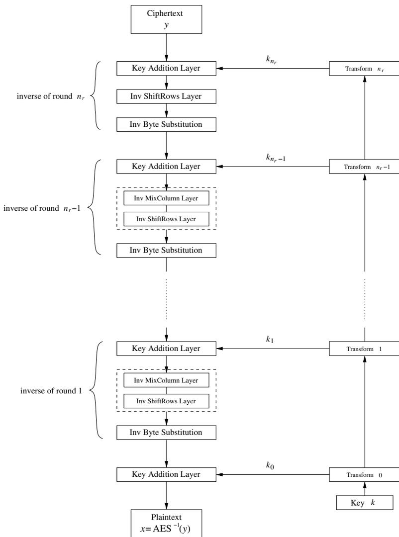
**Fig. 4.8** AES decryption block diagram
