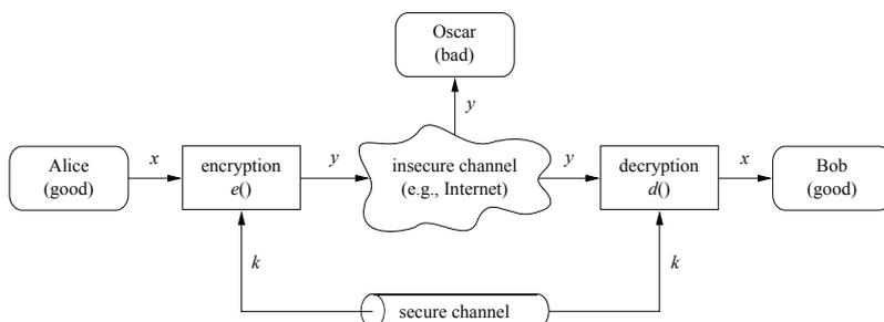
Fig. 1.5 Symmetric-key cryptosystem
