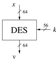
**Fig. 3.3** DES block cipher
