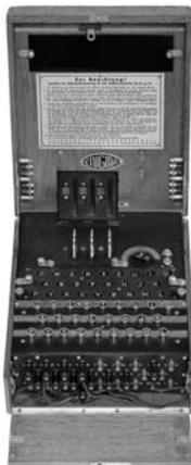
**Fig. 1.1** The German Enigma encryption machine (reproduced with permission from the Deutsches Museum, Munich)
