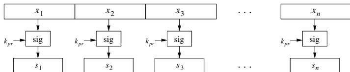
**Fig. 11.1** Insecure approach to signing of long messages
