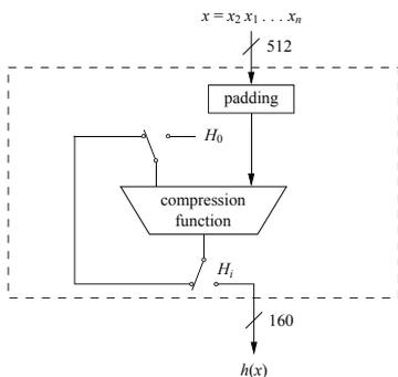
Fig. 11.9 High-level diagram of SHA-1
