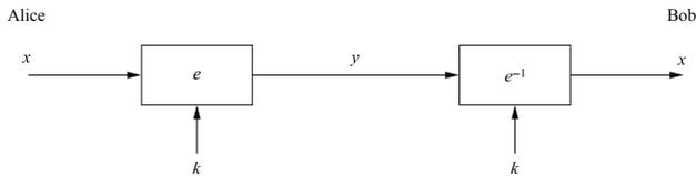
**Fig. 6.1** Principle of symmetric-key encryption
