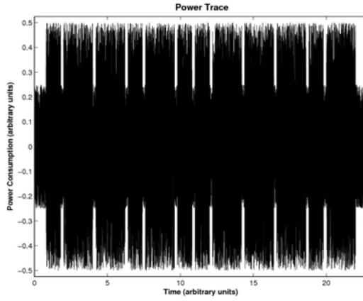
Fig. 7.5 Power consumption of an RSA decryption
