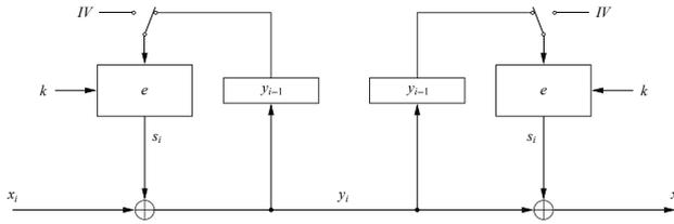
Fig. 5.6 Encryption and decryption in CFB mode
