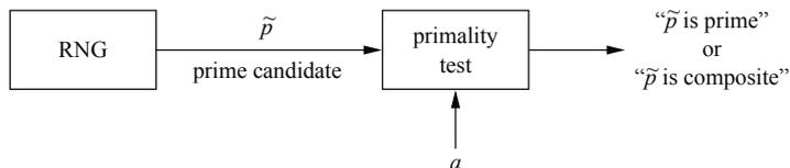
**Fig. 7.2** Principal approach to generating primes for RSA
