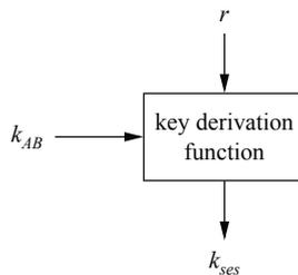
**Fig. 13.2** Principle of key derivation
