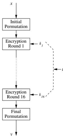
Fig. 3.4 Iterative structure of DES
