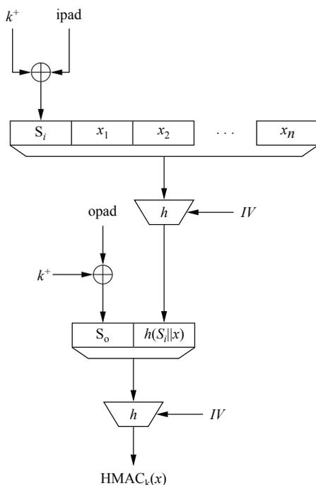
Fig. 12.2 HMAC construction
